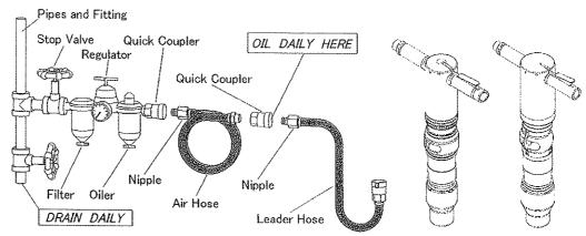
Whether there is any dust, or damage to the air connection portion. Whether the air hose is tight enough.
