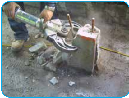
HCS 8 J can crush concrete wall up to 15cm thick.
