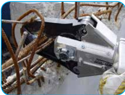
HCS 8 S cuts steel bar of Ø 16mm, and pipe of Ø 50mm x 1.5mm
