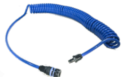
Coil Hose Assembly (2m, 4m, 6m and 8m) -id 5mm x od 8mm -id 6.5mm x od 10mm -Max operating pressure: 10bar
